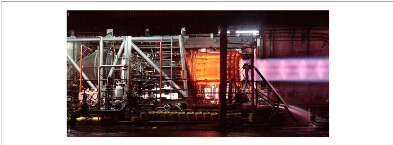
Figure 4. Modern static test with “rain-making machine.” Note. Exiting water is in lower right of the image.
